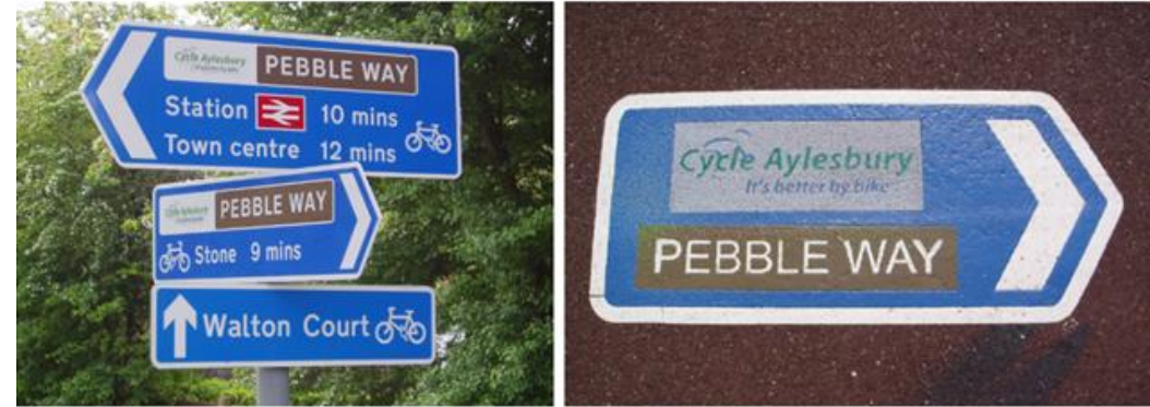
Signage in Aylesbury showing route branding and local destination off the main route & Thermoplastic marking used only off-highway
